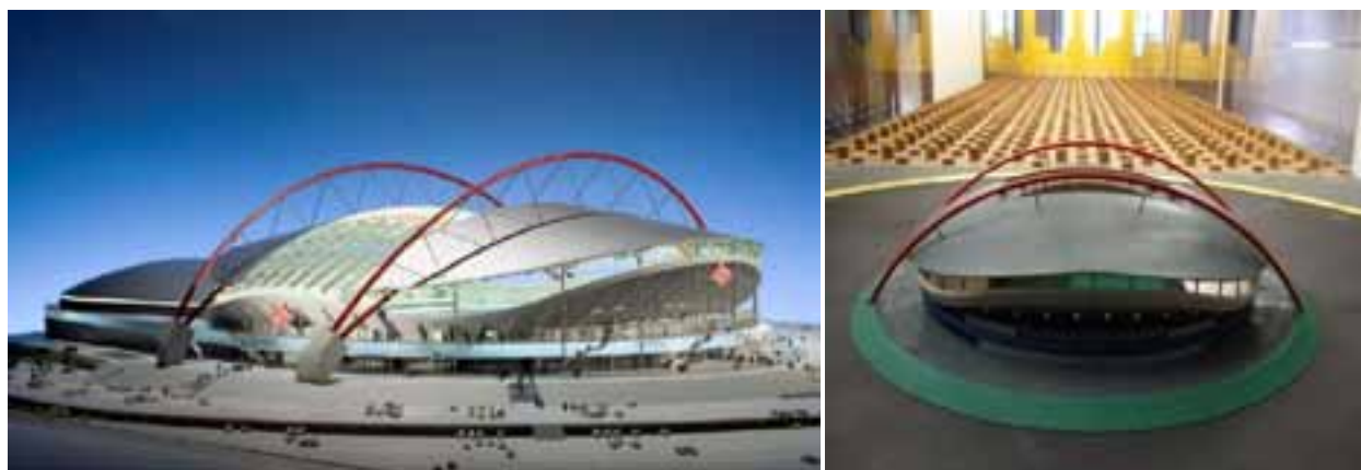
Figure 2.7: Animation of Spartak Moscow Stadium and implemented model at boundary layer wind tunnel, Ruhr-Universität Bochum
